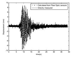
Figure 6 Typical time history comparison between calculated displacements and direct measurement (Bassam, et al, 2011)
