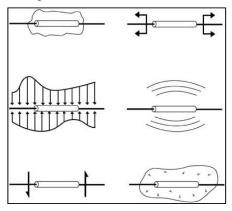
Figure 1 FBG packages for monitoring of structural perturbations (Ansari, 2007).
