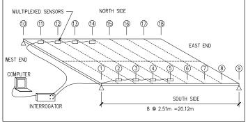
Figure 8 Accelerometer locations on the bridge (Talebinejad, et al, 2009).
