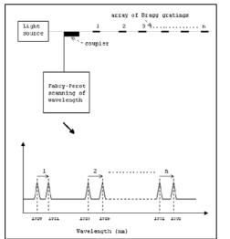
Figure 2Serial multiplexing of FBG sensors (Ansari, 1997).
