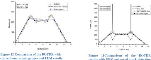
results with FEM enhanced crack detection capabilities (Motamedi, et al, 2012)
