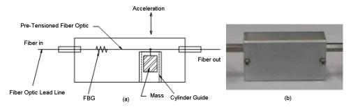
Figure 7; (a) schematic design of the FBG accelerometer; (b) photo of the FBG accelerometer (Talebinejad, et al, 2009).
