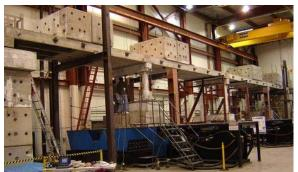
Figure 3 Quarter scale prototype of the four span bridge on shaking tables.
